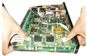
color latching connectors (male) placed at the bottom of the daughter board with the other female connector placed on the Granddaughter and main board. As shown above in Fig. 3.5.2e
